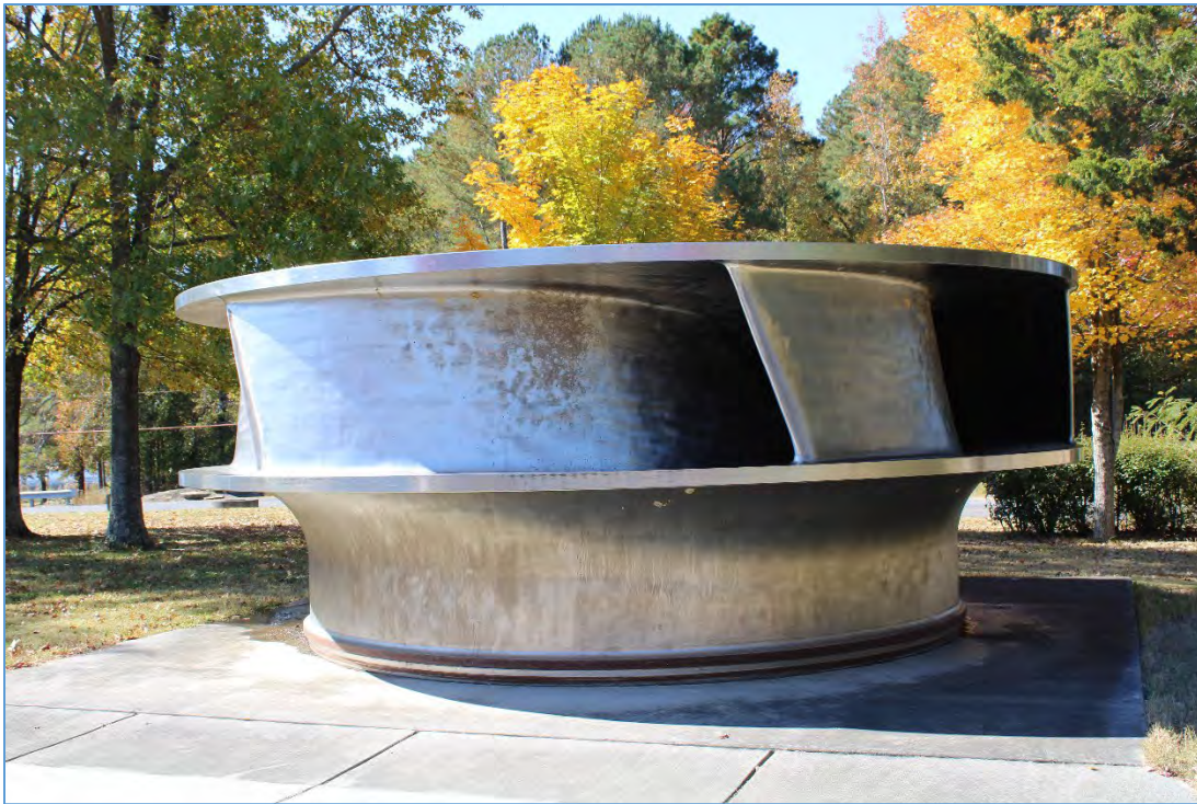
Figure 100: Francis-type reversible pump-turbine impeller located at the Visitor Center, looking west.
